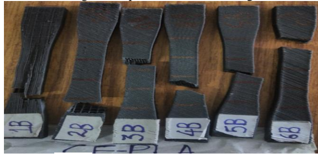
Figure 8. Specimens' failure after testing.
