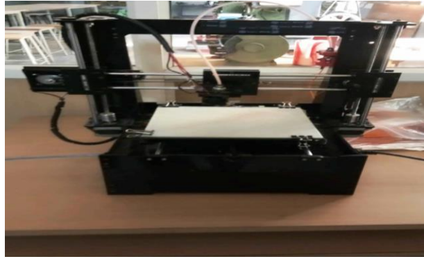
Figure 1. Mechanical part makers FDM 3D printer
