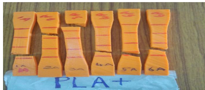
Figure 6. Specimens' failure after testing
